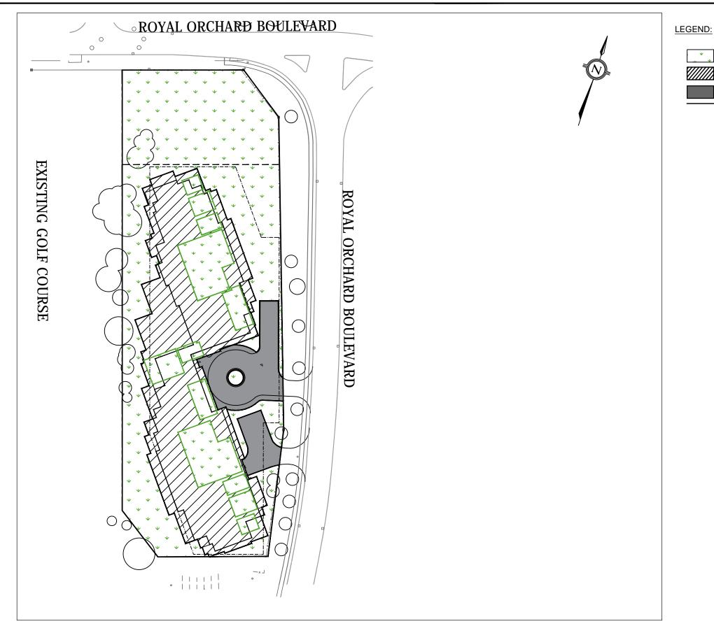
% COVERAGE PERVIOUS AREAS (i=0%) 6553 sq.m. 61 % BUILDING (i=100%) 3210 30 IMPERVIOUS PAVEMENT (i=100%) 10,703 sq.m. (i=39%) TOTAL
