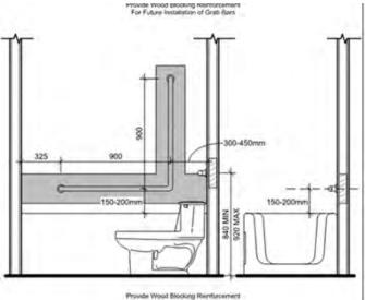
Provide Wood Blocking Reinforcement For Future Installation of Orab Bans
